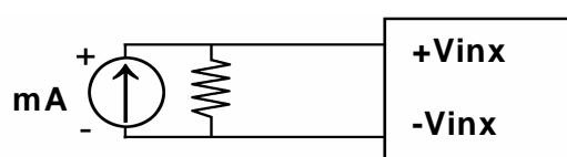
P.S. with 125ohms resistor
