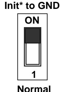
2. Sliding the INIT\* switch to the Init(ON) position of rear side then Power On will enter INIT\* mode (use ASCII command).
