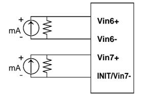
**EX9017F** Analog I/P Channel 6 and 7 wire connection, while the jumper JP1 setting is Init\* mode.
