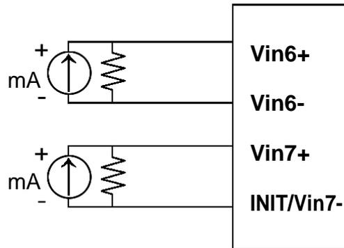
**EX9017F** Analog I/P Channel 6 and 7 wire connection, while the jumper JP1 setting is Init\* mode.
