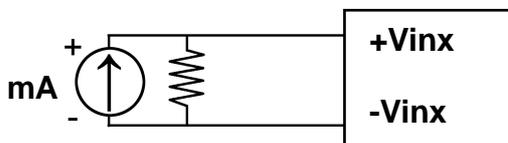
**EX9017/17F** Analog I/P Channel 6 and 7 wire connection, while the jumper JP1 setting is 8 differential mode.
