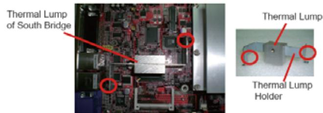
2. Use screw driver to remove the 2 screws. Keep the screws safely for later use.
