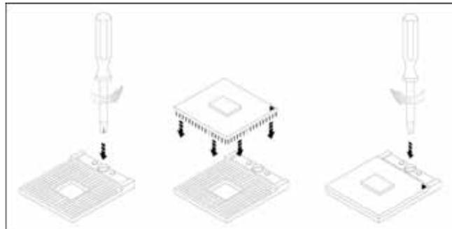
4. Place the CPU into the socket by making sure the notch on the corner of the CPU corresponding with the notch on the inside of the socket. Once the CPU has slid into the socket, lock the screw.
