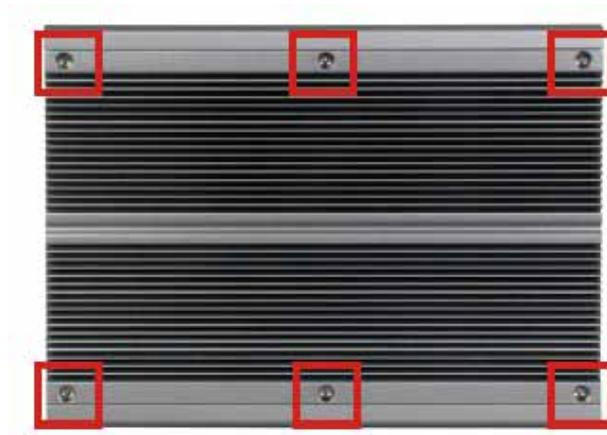
2. Use screw driver to remove the top cover screws. Keep the screws safely for later use.
