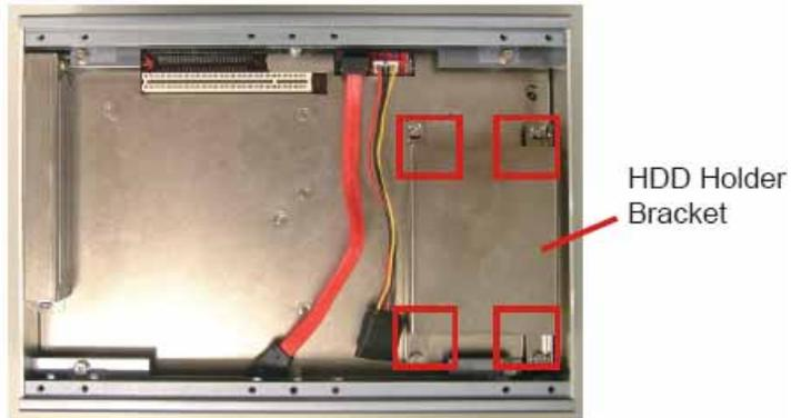
3. Use screw driver to remove the screws. Keep the screws safely for later use.
