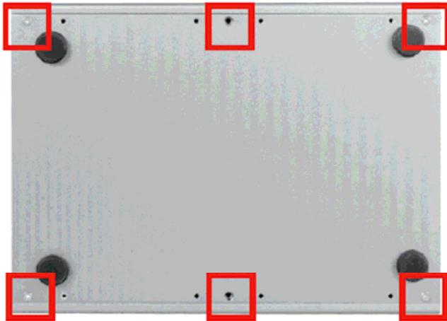
2. Use screw driver to remove the bottom cover screws. Keep the screws safely for later use.
