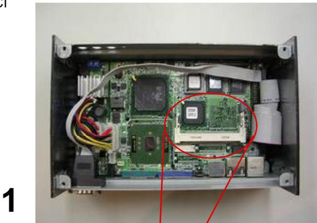
2. Insert and press the Mini PCI card down until it snaps on the latches.
