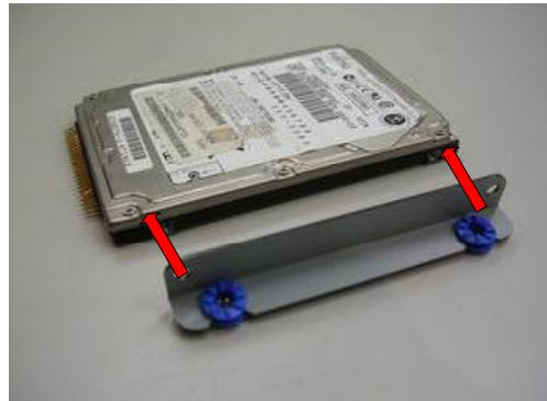
Note: For easy installation, it's recommended to keep the connectors of HDD and mainboard on the same direction.
