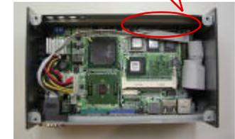
3. Connect the other end of IDE cable to the IDE connector on the drive.
