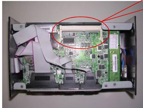
2. Locate the 144-pin SODIMM sockets on the main board of the main unit. Align the SODIMM on the socket and let the notches on the SODIMM meet the break on socket. Firmly insert the DIMM into the socket until the retaining clips snap on and the SODIMM is properly positioned.
