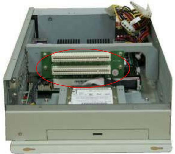
Now slide the addon into the PCI slot, making sure the golden part faces the slot. When both parts that are interfaced together come into the right contact, slightly push the addon into the rail of the slot. This shows the addon is already completely connected.
