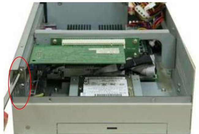
To finish the job, just fasten the 8 screws as shown in the picture.
