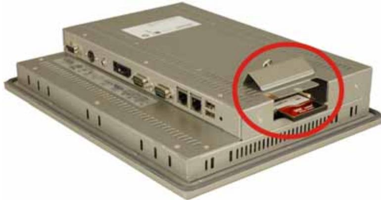
**Figure 3-1: CF Card Installation**
