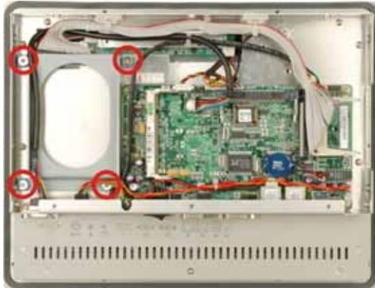
**Figure 3-7: HDD Bracket Retention Screws**
