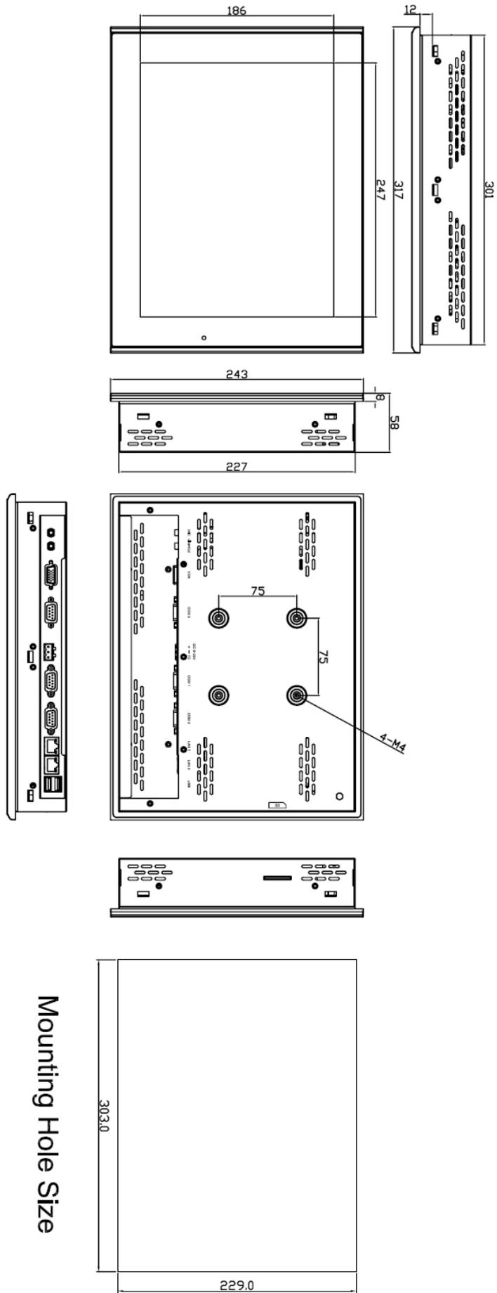
**Figure 1.4: Dimensions of the EX-96123-A**
