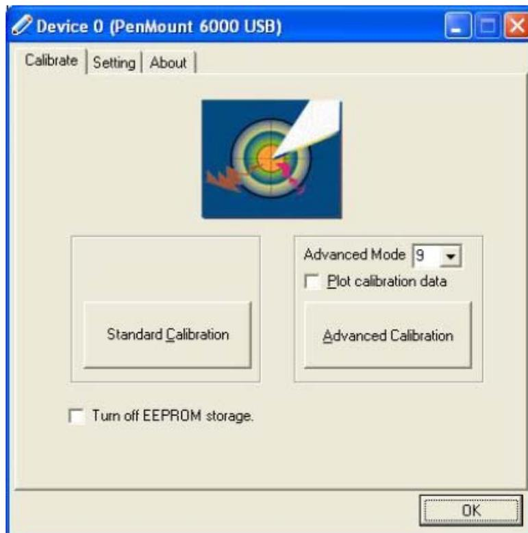
**NOTE:** Recommend to use a stylus during Advanced Calibration for greater accuracy.
