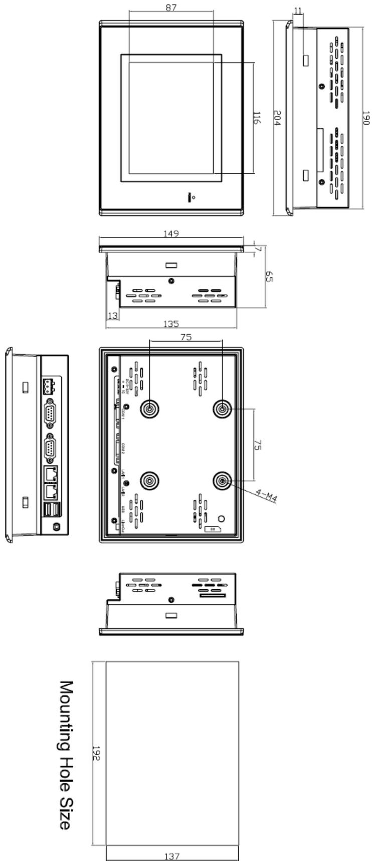
**Figure 1.1: Dimensions of the EX-96053-A**
