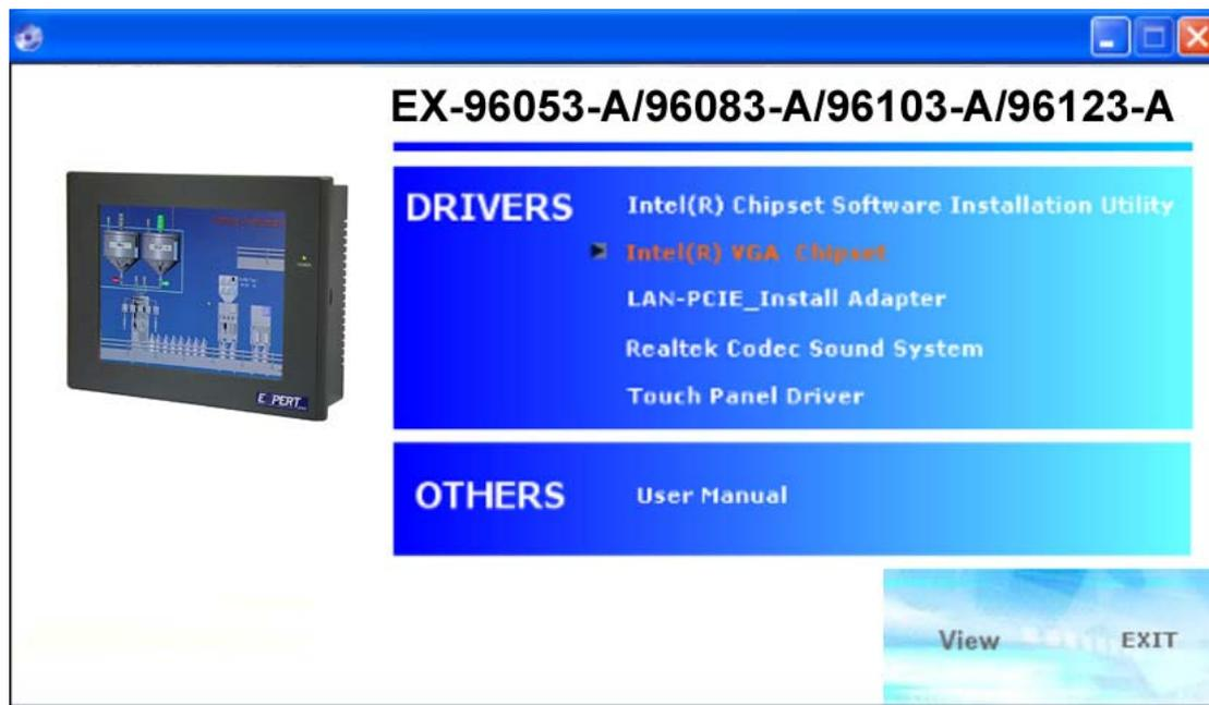
Follow the step-by-step installation process to install the Graphics Media Accelerator driver.
