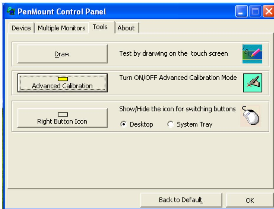
Select “**Device**” to calibrate, then you can start to do “Advanced Calibration”.
