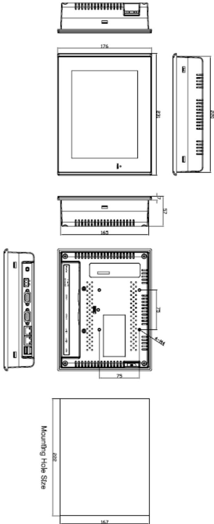
**Figure 1.2: Dimensions of the EX-96083-A**
