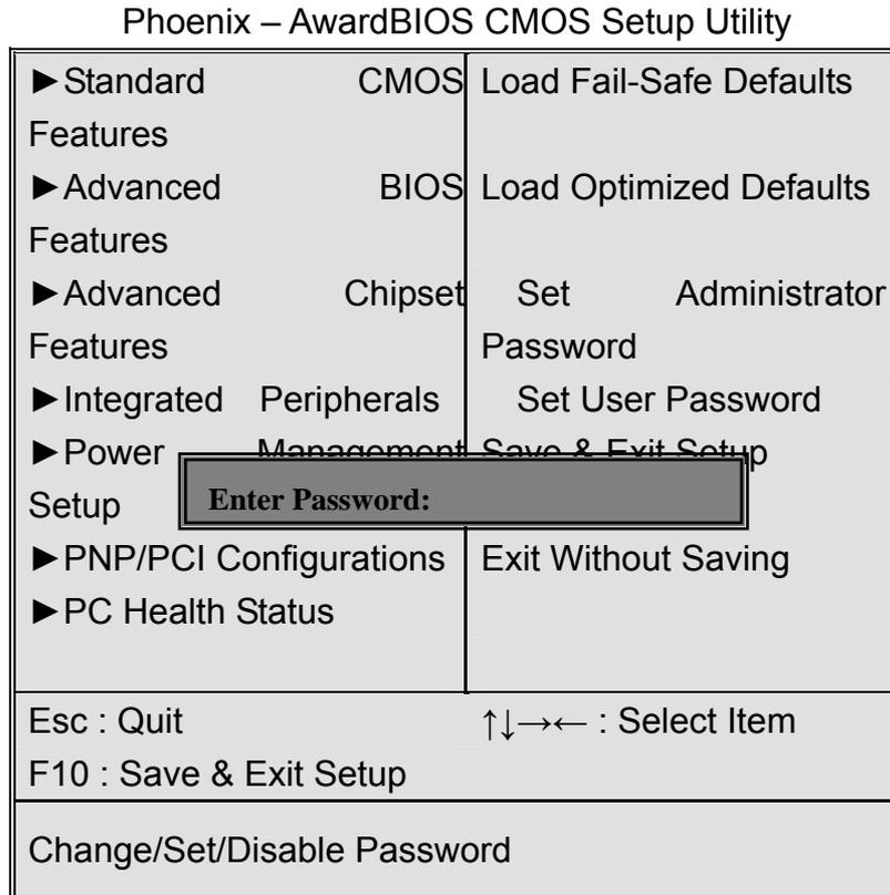
Type the password with up to 8 characters and then press <Enter> key. This will clear all previously typed CMOS passwords. You will be requested to confirm the password. Type the password again and press <Enter> key. You may press <Esc> key to abandon password entry operation.
