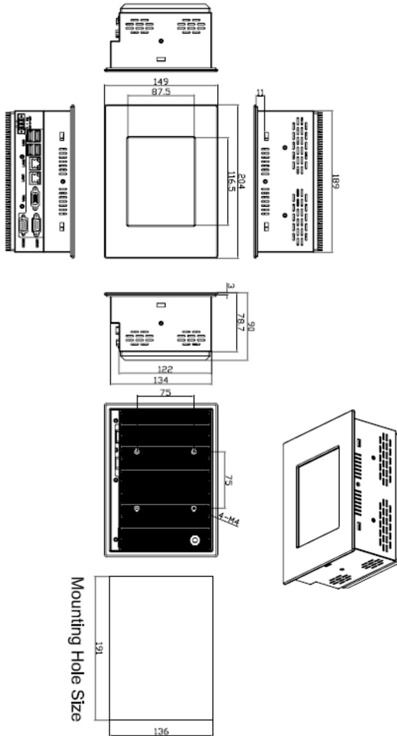
Figure 1.1: Dimensions of EX-96057A
