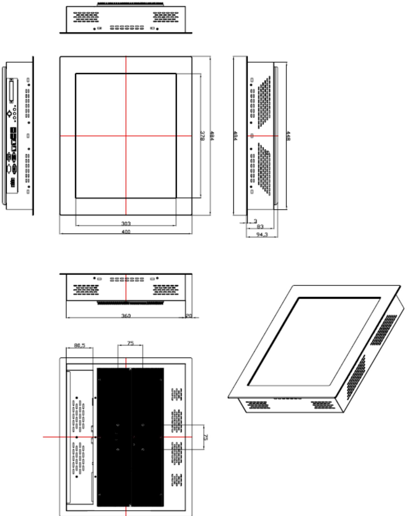
**Figure 1.7: Dimensions of the EX-96197A**
