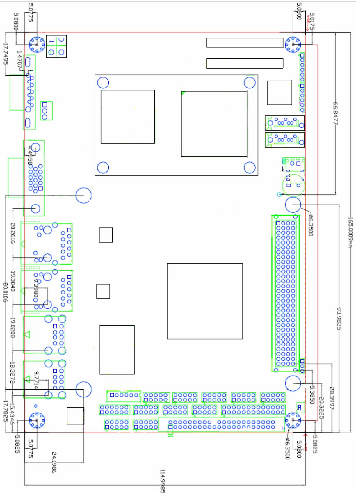
**Figure 2.2: Mainboard Dimensions**
