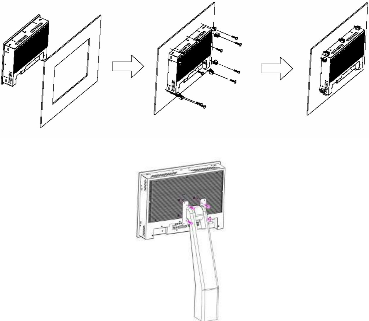
**Figure 1.10 Panel mounting and VESA mounting of the EX-96XX7A**
