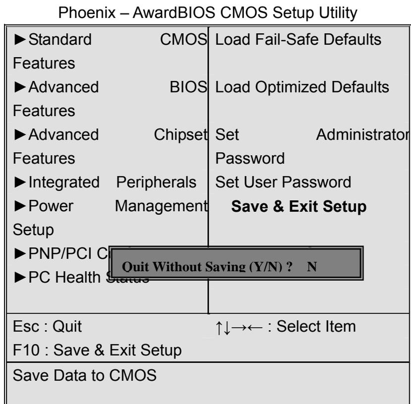
Press **Y** and then **Enter** key to exit from BIOS setup without saving the changes.
