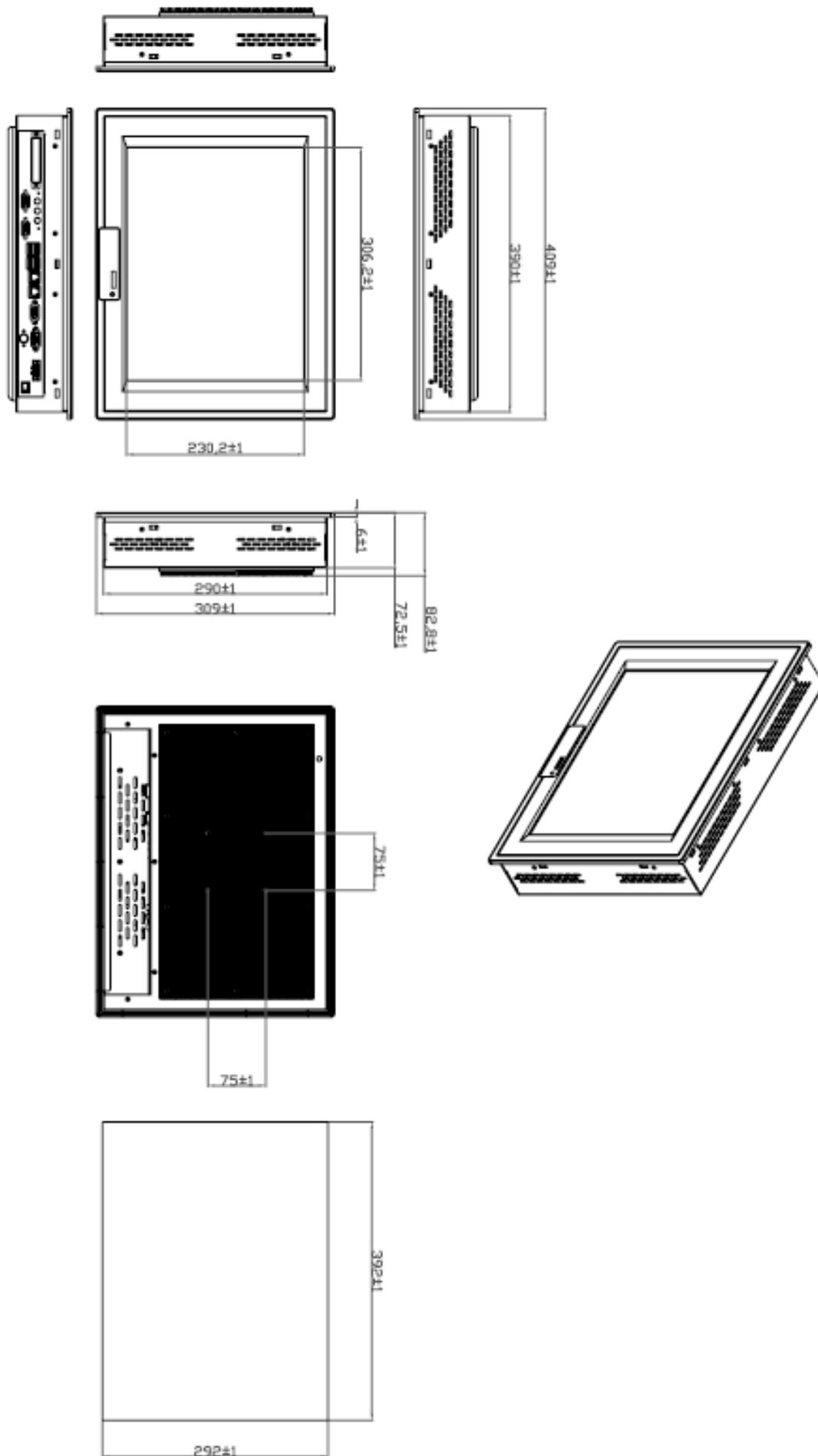
**Figure 1.5: Dimensions of the EX-96157A**
